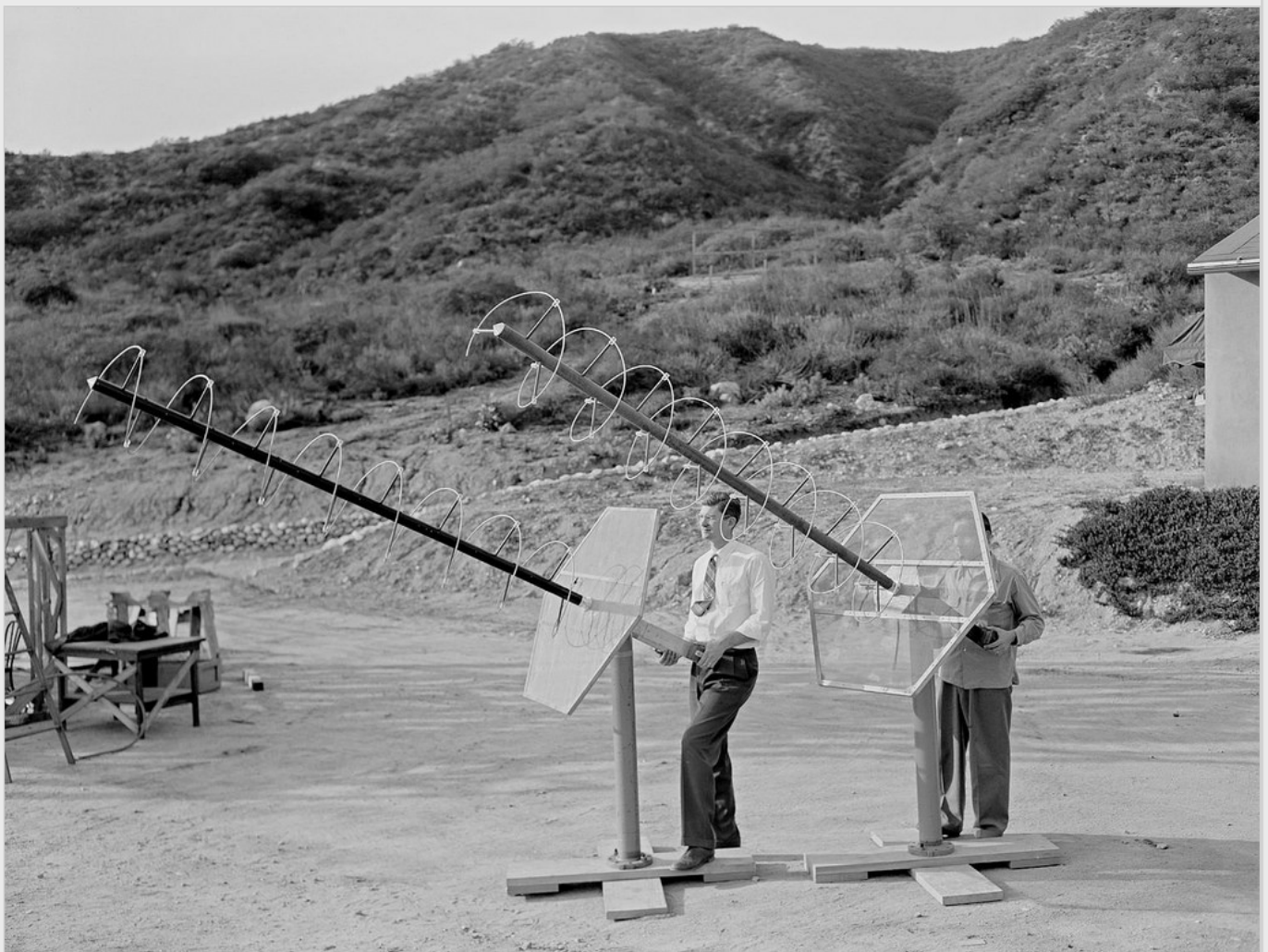
Helical beam antennas from 1951.
